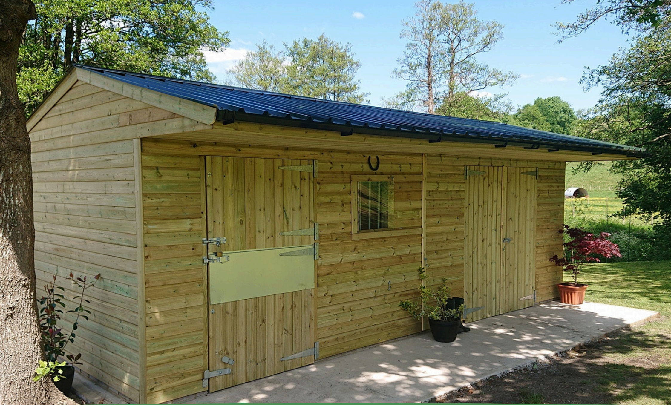
A Beautiful setting for a 3.6x7.2m Stable and store from our Exmoor Specification Bolted to a course of semi engineering bricks and a 150mm Concrete foundation
